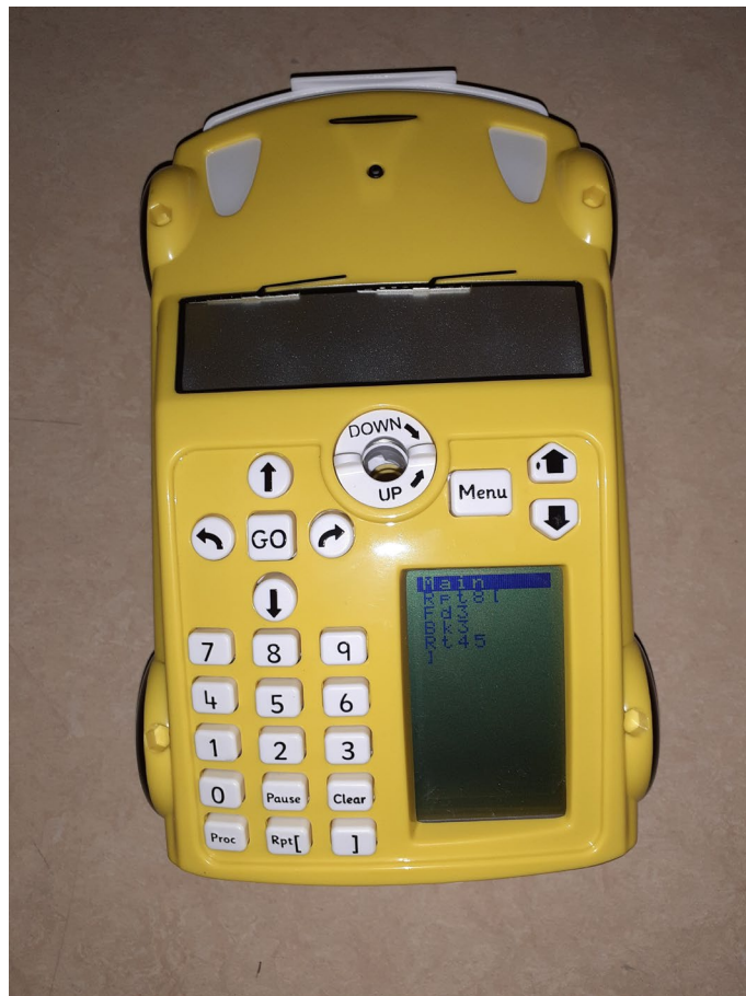
Figure 3.1 The keyboard and screen of Pro-Bot .
