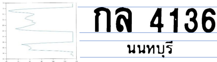
Figure 2.4.5 The histogram of accumulated values in each row
