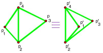
The above construction is globally rigid on a plane and is not globally rigid in the space.
