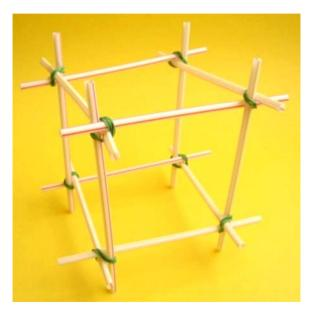
Now, by joining ends of bars by cables in such a spatial woven structure one may obtain examples of polyhedral tensegrity structure. In each case they appear in two versions L and R.
