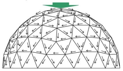
From the point of view of forces acting on tensegrity structures, we may divide them in categories. In one category there are frameworks made up of rigid bars. The bars making up the construction are connected in polygons, mostly triangles, sometimes pentagons or hexagons. Each bar is oriented.
