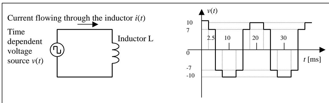
Figure 2 The electrical circuit and the applied voltage function  $v(t)$
