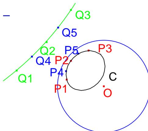
**Figure 3.2** Construction of the orthogonal projected image of a small circle.
