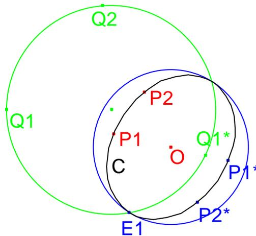
**Figure 3.1** Construction of the orthogonal projected image of a great circle.
