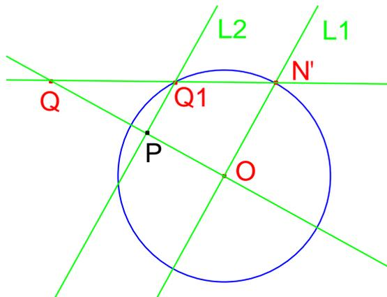
**Figure 2.2** Construction of the orthogonal projected point from a stereographic projected point.
