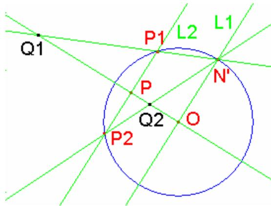
**Figure 2.1** Construction of stereographic projected points from an orthogonal projected point.
