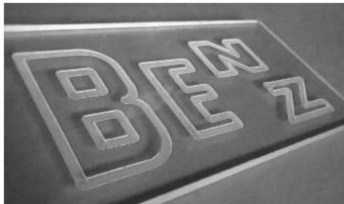
Figure 4.6 A finished workpiece created by a CNC milling
