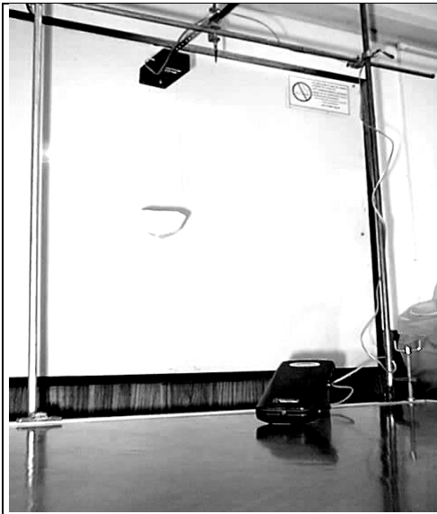
Figure 1. Experimental arrangement for the body's velocity and displacement registration.
