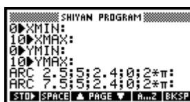
Create two circles on both left and right sides; , we need to divide the circle into 12 parts and indicate the scale. The HP39gs only has a function of line drawing. So we calculate the coordinate of these 12 points of parts with the following formula :
