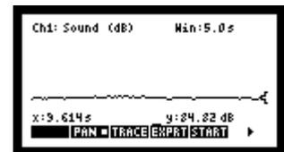
As soon as the ‘Sound’ tool starts, there will be a ‘strip curve’: appearing on the screen of HP39gs with little variation, though, which is due to the excessively-dense data collection. Now we need some ‘finer’ graphics. So we can press the key ‘zoom’, together with the direction keys ‘+’, ‘-’ for the amplification and narrowing of the graphics (when the ‘zoom’ key works, ‘ZOOM’ will turn to ‘ZOOM’. There will be a direction for the special function of the ‘pan’ key in the following table.)
