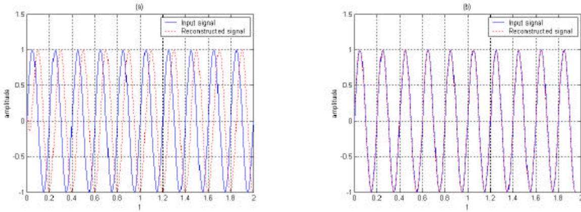
Fig 5. (a) The signal reconstructed by  $h_o(z) = \frac{\bar{b}(z)}{a(z)}$  (b) With system delay  $L=5$ , the reconstructed signal and the input signal.
