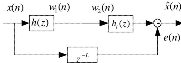
Fig 3. The proposed stable inverse system structure.
