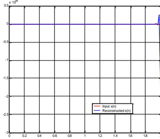
Fig 2. The signal  $x(t) = \sin(2\mathbf{p} \cdot 5t)$  and reconstructed signal by the inverse system
