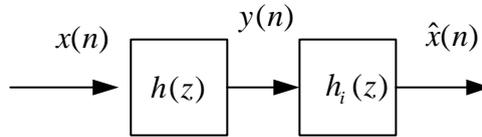
Fig 1. Cascade of a discrete-time system  $h(z)$  with its inverse discrete-time system  $h_i(z)$ .
