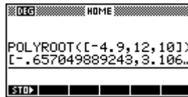
Figure 4. Solving 10 + 12t - 4.9t^2 = 0 to yield the x intercept of the graph in Figure 3.
